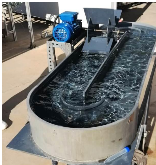
Figure 6- Raceway Pond reactor
